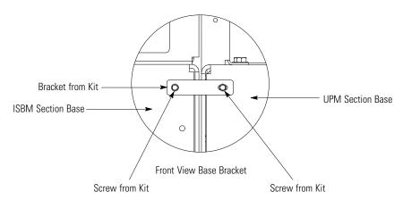
Figure 4-7. ISBM Section to UPM Section Joining Brackets
